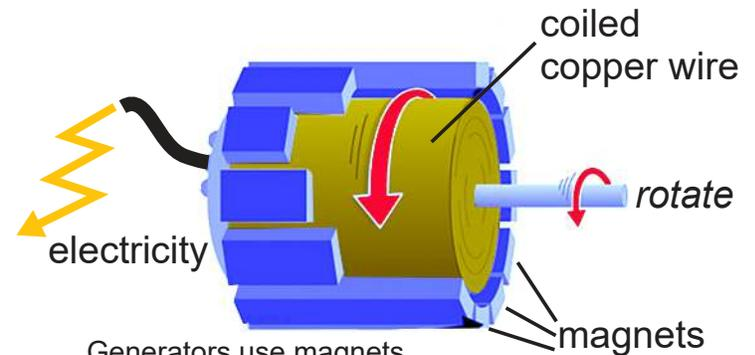
Generators use magnets and motion to make electricity
