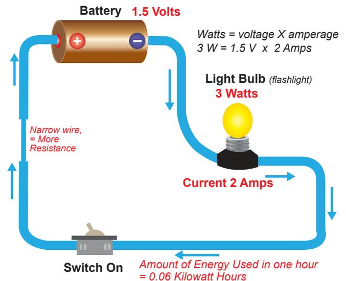
the thickness of the conductor wire will increase the amount of electricity that can travel along it. Resistance is measured in **Ohms**.
