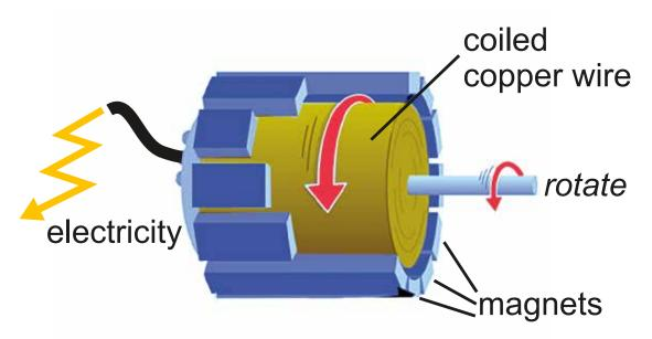
**Generators use magnets** and motion to make electricity.
