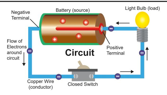
Batteries convert chemical energy into electricity.
