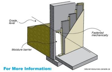
Keeping The Heat In - Section 6: Basement insulation: floors, walls and crawl spaces- Natural Resources Canada
